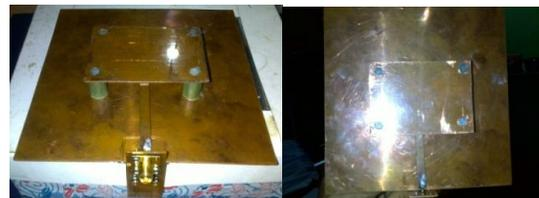
Gambar 7. Hasil Prototipe Antena mikrostrip *patch rectangular*
